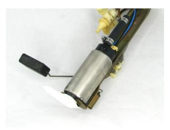
5 – reinstall the assembly into the fuel tank and attach a length of hose to the outlet of the pump assembly allowing it to drain into a fuel safe container and prime the fuel pump assembly
