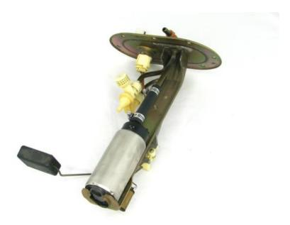
4 – install the fuel sock and plug in the electrical connector
